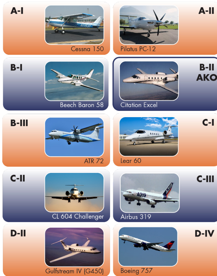
FIGURE 4-1: RUNWAY DESIGN CODE (RDC)
