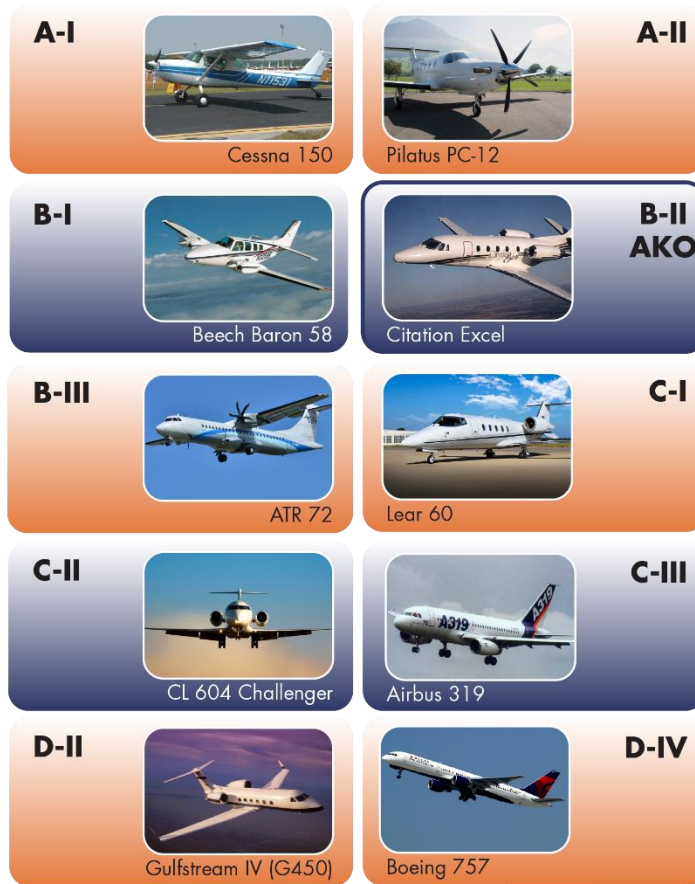
FIGURE 4-1: RUNWAY DESIGN CODE (RDC)
