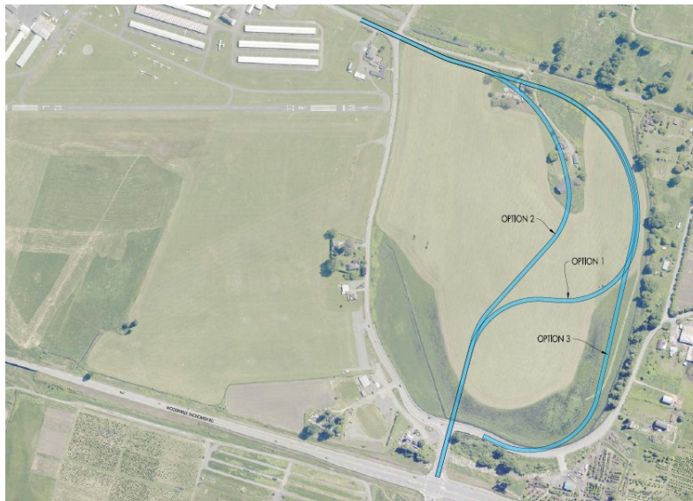
FIGURE 6-5 – AIRPORT WAY RELOCATION OPTIONS
