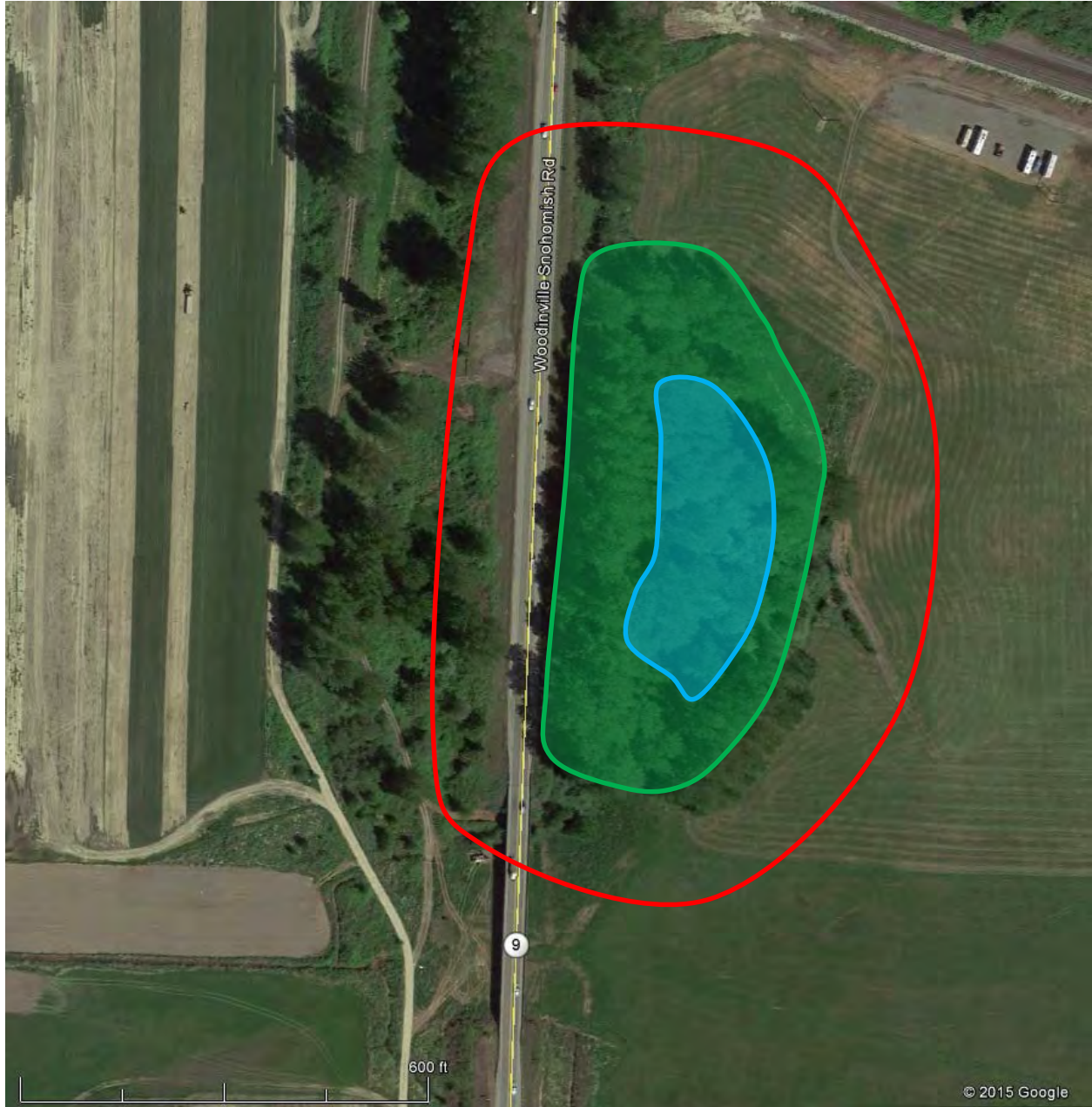
Figure 2. Hydrology: hydroperiods, outlets, and 150ft buffer - D1.1, D1.4, D4.1, H1.2, D2.2, D5.2
