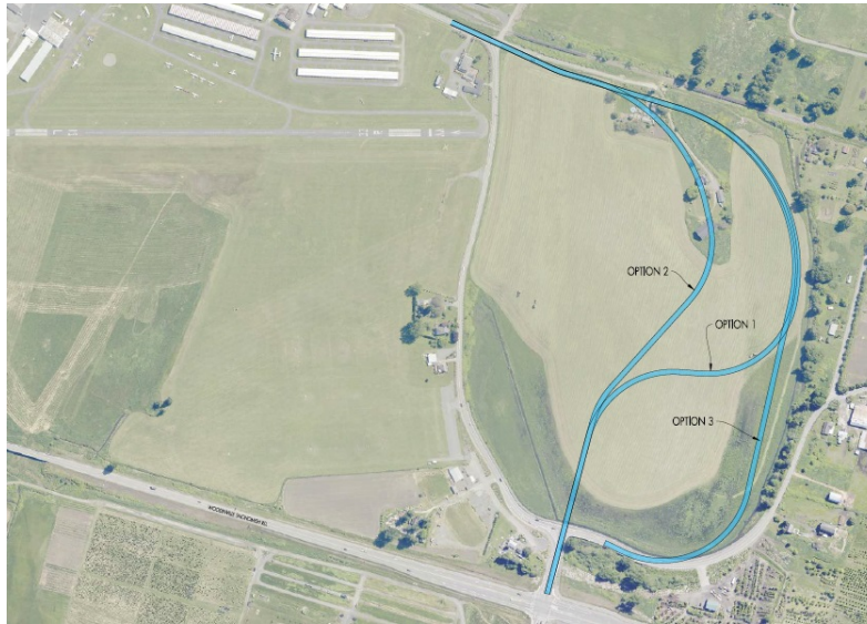
FIGURE 6-5 – AIRPORT WAY RELOCATION OPTIONS
