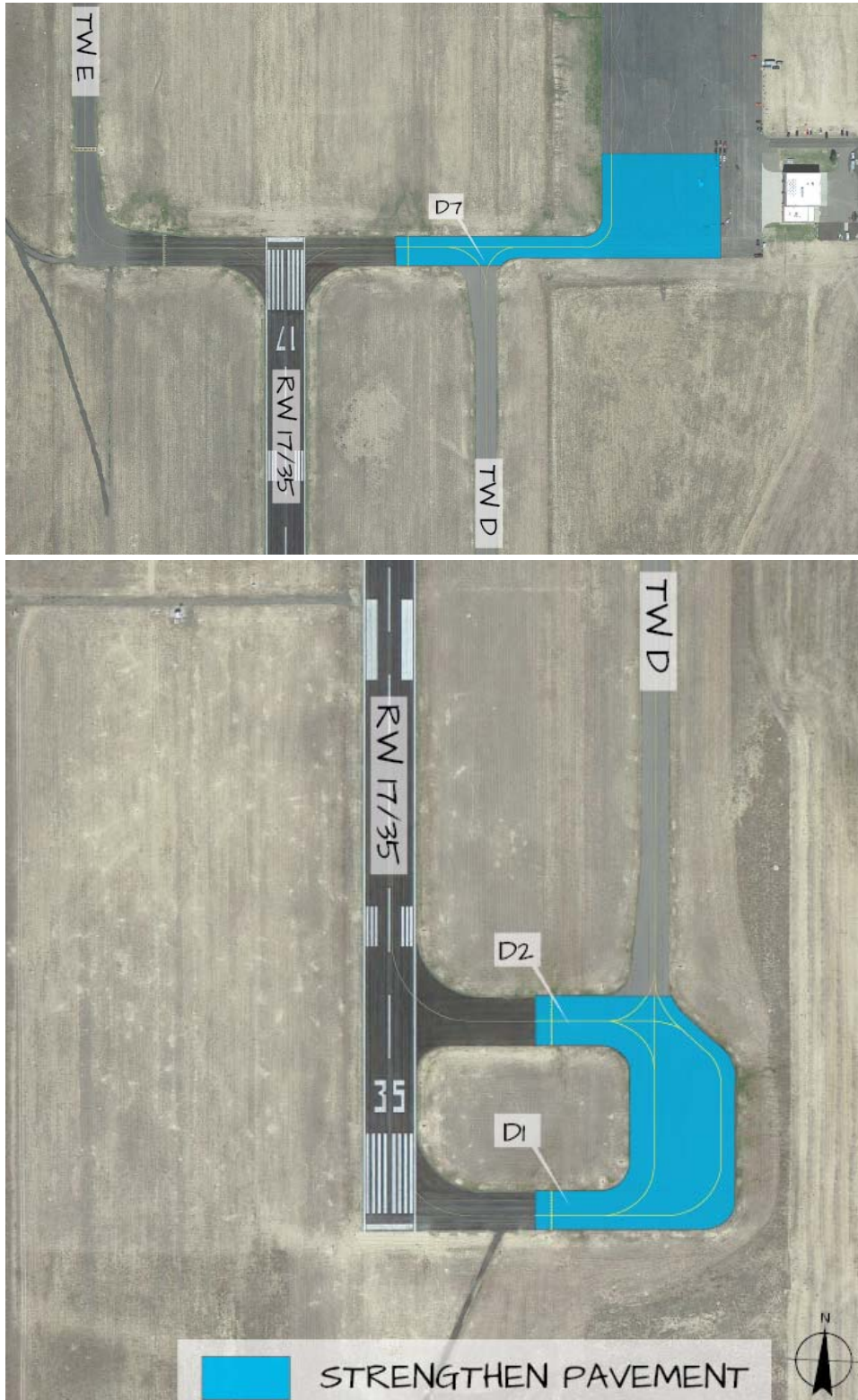
FIGURE 5-8 - TAXIWAY STRENGTHENING AT FTG
