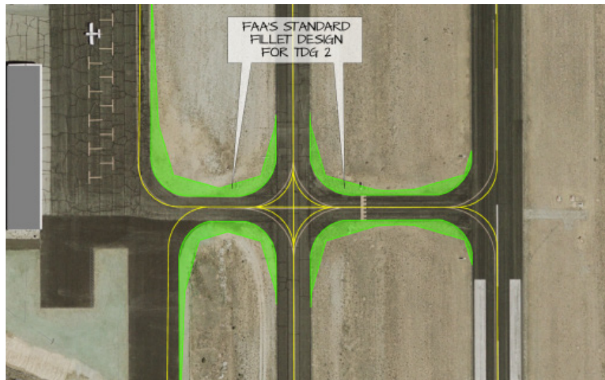
FIGURE 4-5 – FAA TAXIWAY DESIGN GROUP 2 FILLET DESIGN REQUIREMENTS
