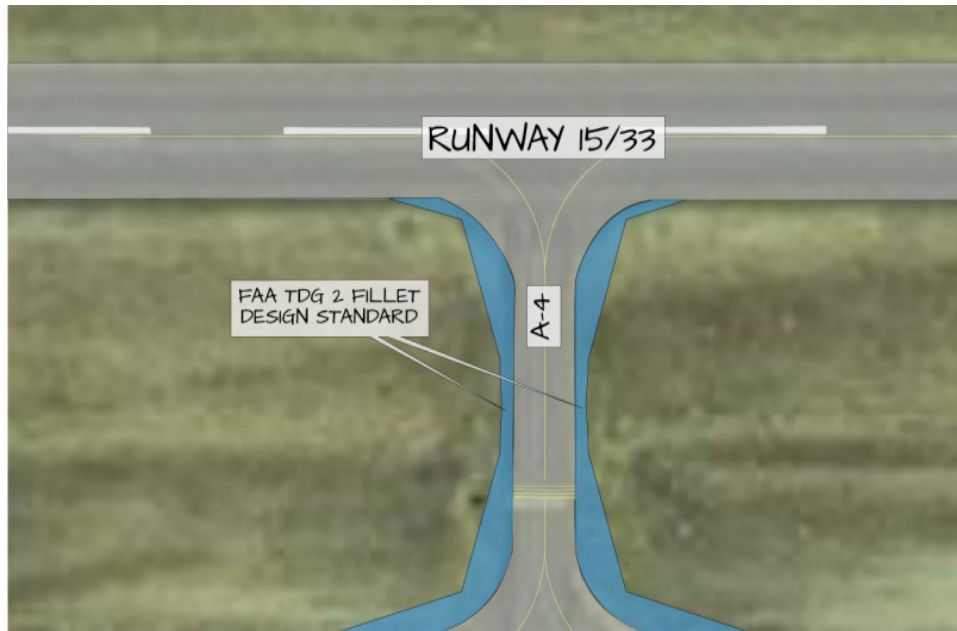
FIGURE 5-3 - FAA TAXIWAY DESIGN GROUP (TDG) 2 FILLET DESIGN REQUIREMENTS
